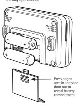
If you have followed all of the above steps correctly, your unit will begin monitoring for CO in around 3 minutes. When the 3 minute warm-up period is complete, the Power LFD will flash green once per minute to indicate that the alarm is receiving power from the batteries and is fully operational (if your detector chirps or enters alarm following the 3 minute warm-up period and your product is still within warranty, then please contact technical support for advice).
