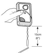
Step 5 After step 4, put out the incense stick or cigarette by placing it into a dish of water. Ensure that all flames have been extinguished.
